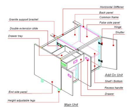
Laboratory Work bench comprises of following components:
