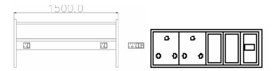
The service panels carry all electrical fittings and are attached with Reagent shelf. It comes in the modular range of Reagent shelves.
