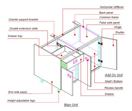
Laboratory Work bench comprises of following components:
