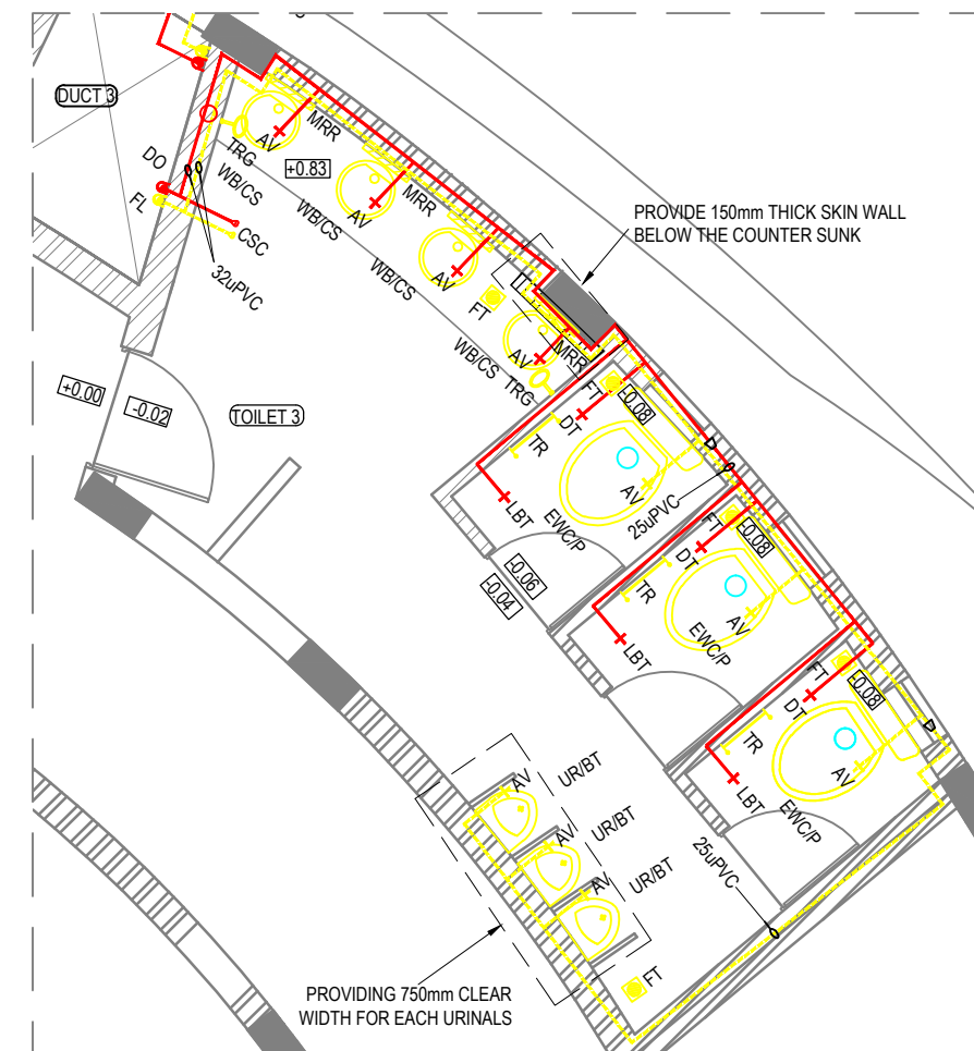
PLUMBING LAYOUT SHOWING WATER SUPPLY LINES IN TOILET 3 IN GROUND FLOOR SCALE 1:30
