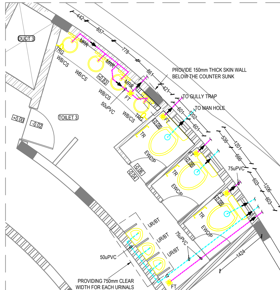
PLUMBING LAYOUT SHOWING WASTE LINES IN TOILET 3 IN GROUND FLOOR SCALE 1:30
