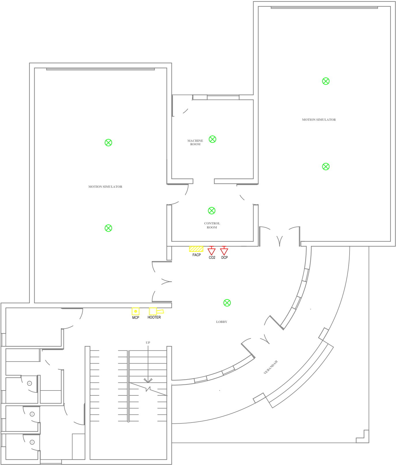
GROUND FLOOR PLAN SHOWING FIRE SUPPRESSION ARRANGEMENTS SCALE 1:50
